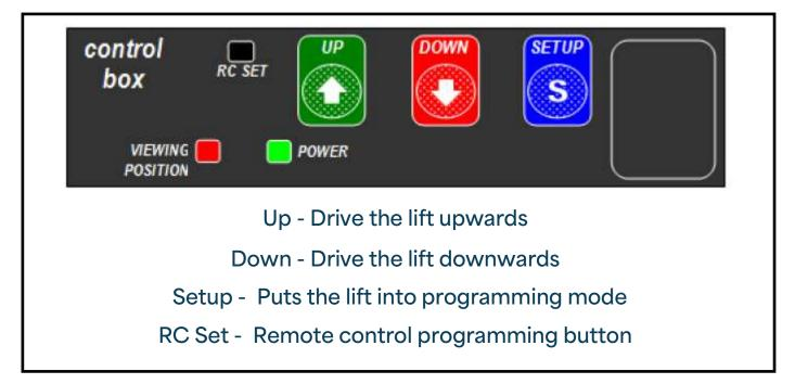
After setting the box up and connecting all sockets the control box will than perform a self test. Successful completion of the self test will be symbolised by 3 short beeps and a flash of the red LED.
